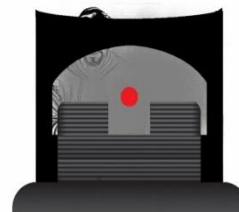
IF PHORIA OCCURS, DOMINANT EYE PROVIDES ALL DATA, PREVENTING BINOCULAR VISION. AS OPTIC IS ALIGNED WITH DOMINANT EYE, TARGET IS OBSCURED.
